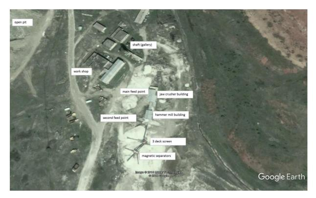
Figure 12-4 Magnesite dry/wet processing plant, location identified during site visit March 2019
