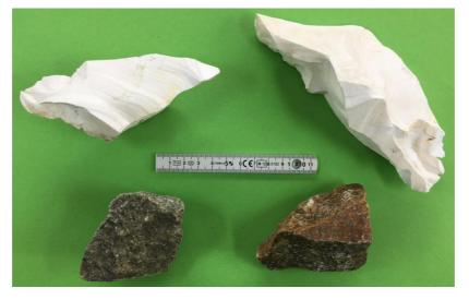
Figure 12-24 Samples of ROM material magnesite and dunite
