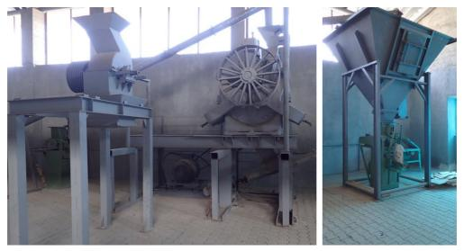
Figure 12-12 Small crushers for special products (left) and packing station (right)
