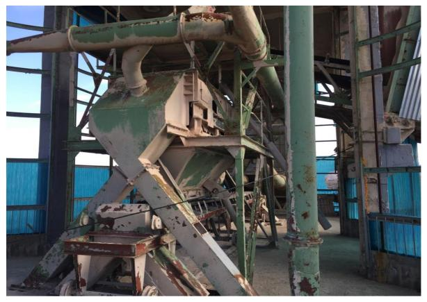
Figure 12-14 Product divider on top of the silo section
