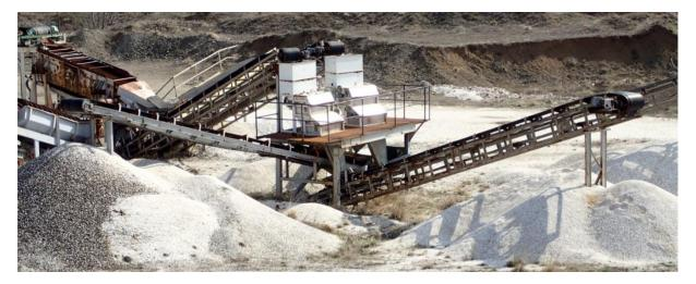
Figure 12-7 Screening and magnetic separation section of the processing plant
