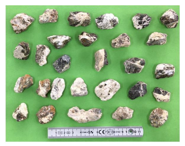
Figure 12-33 Example for non-libarated particles
