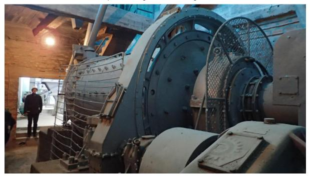
Figure 12-11 Ball mill for MgO flour production
