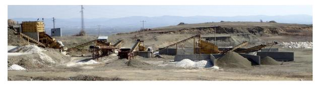
Figure 12-10 Dunite dry processing plant in March 2019
