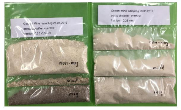
Figure 12-29 Products of magnetic separation of fraction 0.25 - 0.5 mm < 0.25 mm mm (screw classifier overflow)
