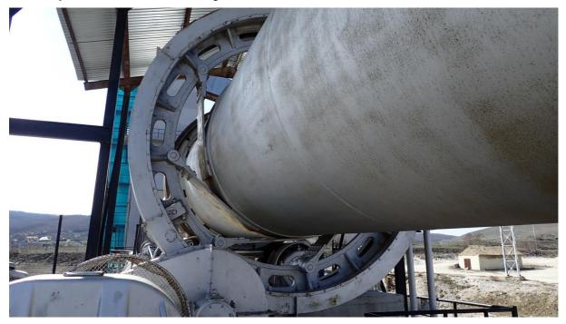
Figure 12-16 Middle section of rotary kiln
