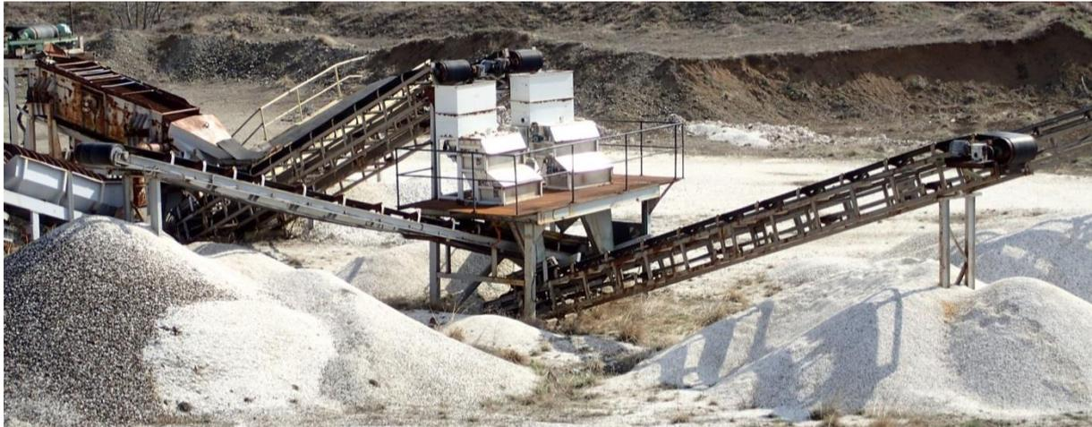
**Figure 12-7 Screening and magnetic separation section of the processing plant**
