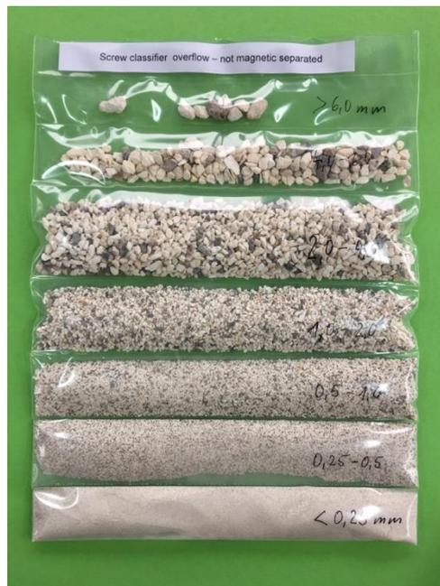
**Figure 12-26 Fractions (PSD) of screw classifier overflow**
