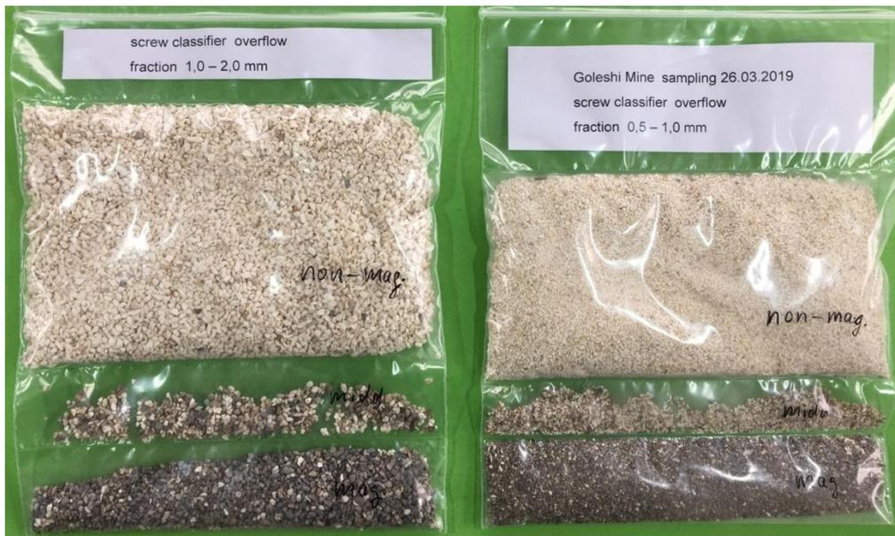
**Figure 12-28 Products of magnetic separation of fraction 1.0 – 2.0 mm 0.5 – 1.0 mm (screw classifier overflow)**
