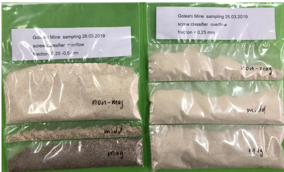
**Figure 12-29 Products of magnetic separation of fraction 0.25 - 0.5 mm < 0.25 mm (screw classifier overflow)**
