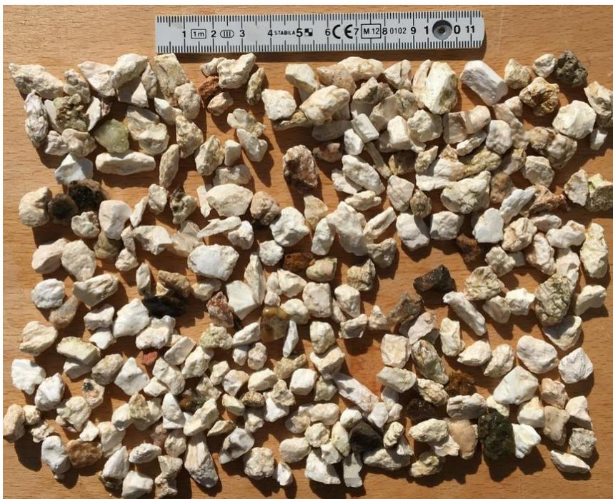
**Figure 12-35 Non-magnetic (magnesite) product from magnetic separation in processing plant, 2 – 15 mm**
