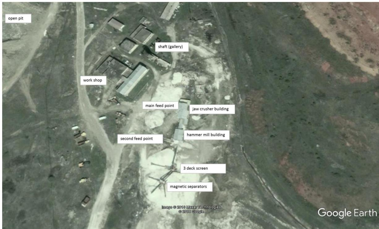
**Figure 12-4 Magnesite dry/wet processing plant, location identified during site visit March 2019**
