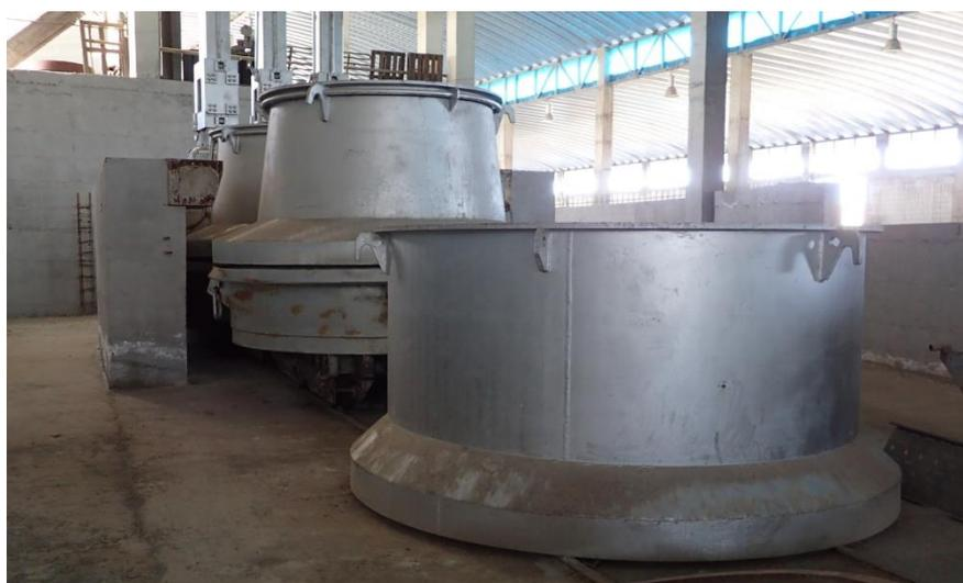
**Figure 12-22 Electrical kiln**
