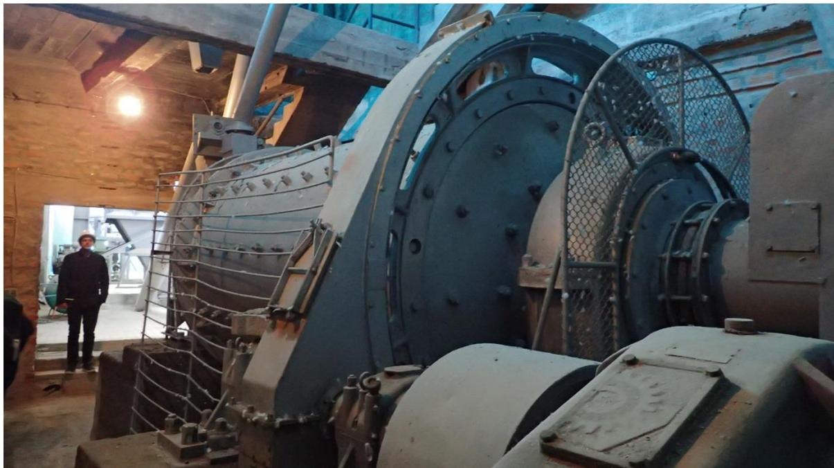
**Figure 12-11 Ball mill for MgO flour production**
