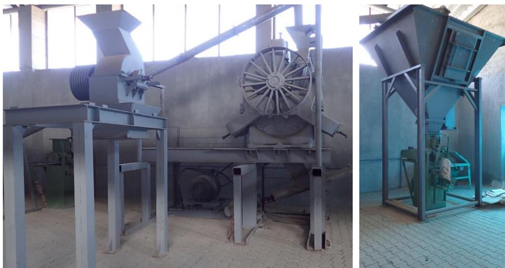
**Figure 12-12 Small crushers for special products (left) and packing station (right)**
