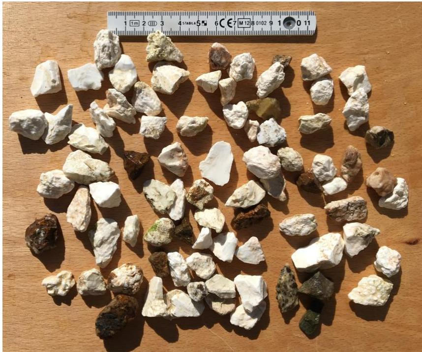
**Figure 12-34 Non-magnetic (magnesite) product from magnetic separation in processing plant, 15 – 20 mm**
